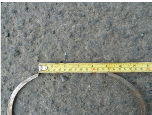
Repair information - calipered outside diameter of main 126mm
