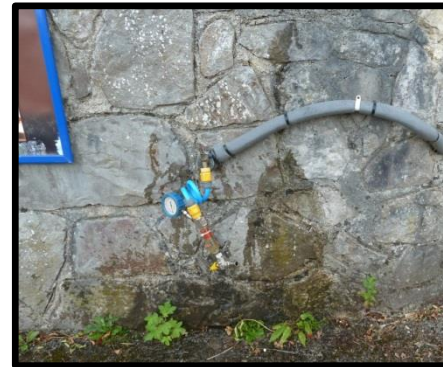
Picture 5 – Pressure & Flow testing equipment
