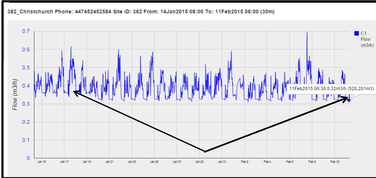
You can see from the above data logger snapshot that the minimum flow rate never drops below approx. 0.32m<sup>3</sup> per hour showing that there is unaccounted water loss on site. This has been ongoing for some time as you can see on the above snapshot.
