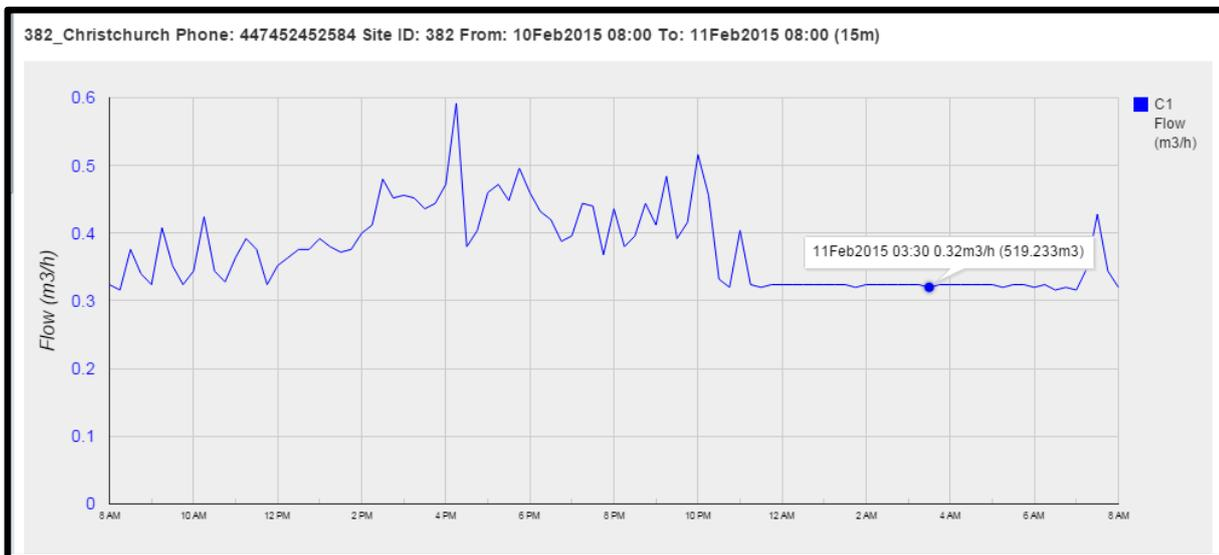
Snapshot of water data logger over last 24 hours. You can see the varying flow rate whilst the site is in use throughout the day and once the site closes at approx. 10.30 pm, there is no variation in flow rate as nothing is being turned on and off, but there is a constant flow of water running throughout the night from a source of approx. 0.32m<sup>3</sup> per hour.
